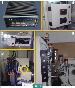
IIoT Hardware integrated on a machine (1 - Edge Device for Data Acquisition, Data Pre-processing, and Cloud Connectivity, 2 - PLC for Data collection from Hardware, 3 - Vibration Sensors for condition monitoring of Wheel Head and Work Head, 4 - Energy Meter for Monitoring Energy Consumption, 5 - Hydraulic Pressure, Pneumatic Pressure, and other IO-Link Sensors for Process and Health Monitoring)
