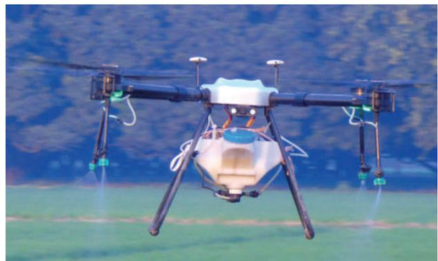
MGT Drone sprinkling pesticides in a potato field
