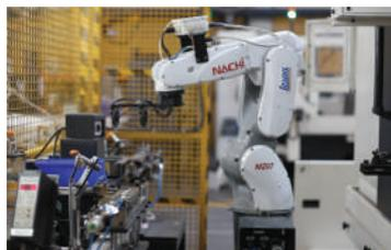
A robot placing a component in front of vision camera for inspection
