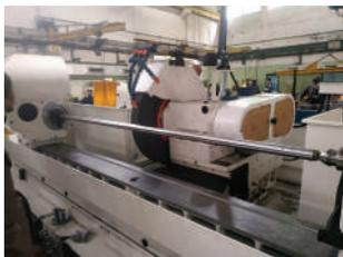
Schenck Guide-rod being finish ground on MGT machine model GCH 440X1200
