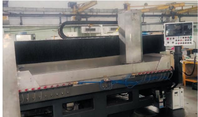
CNC Glass Edge-Milling & Grinding machine built by MGT
